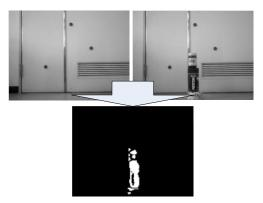
Fig. 6. Background subtraction method, left-top is background image and right-top is current image. Background subtraction method will obtain black-white image (bottom)
