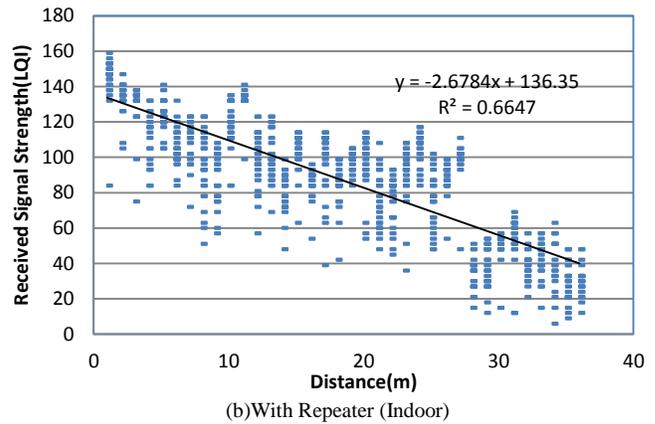
Fig. 21. Example of relation between receiving signal strength and the distance
