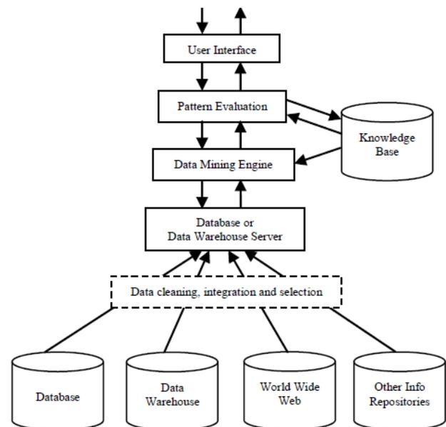
Fig. 1: Architecture of a Typical Data Mining System [1]
