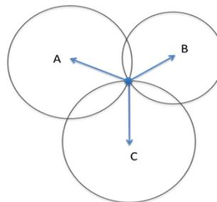
Fig. 18. Location determination concept with three ZigBee stations
