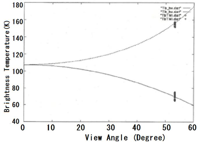
Fig. 2. Brightness temperature for both horizontal and vertical polarizations derived from the proposed physical model based method and actual received brightness temperature with TRMM/TMI of 10.65 GHz of frequency channel acquired on June 2 1998
