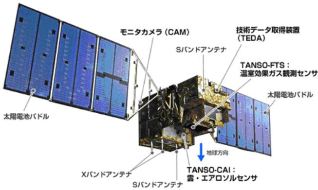
Fig. 1. Mission instruments onboard GOSAT satellite
