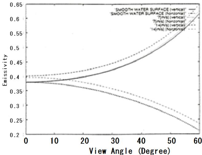
Fig. 1. Emissivity model originated from the Wilheit model
