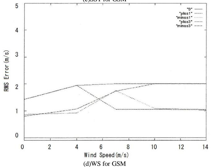
Fig. 3. RMS error of SA and GSM for the estimation of SST and WS with the designated bias of plus minus 1(K), 5(K) for SST and plus minus 1(m/s), 3(m/s) for WS as well as without any bias
