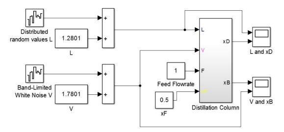
Fig. 3: MATLAB/Simulink model of the distillation column
