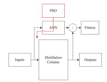
Fig. 2: Schematic diagram of the proposed hybrid system
