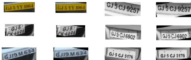
Figure 15 (a) Positive Skew Correction (b) Negative Skew Correction
