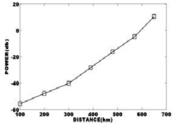
Figure 4: power vs. distance for 32 channels
