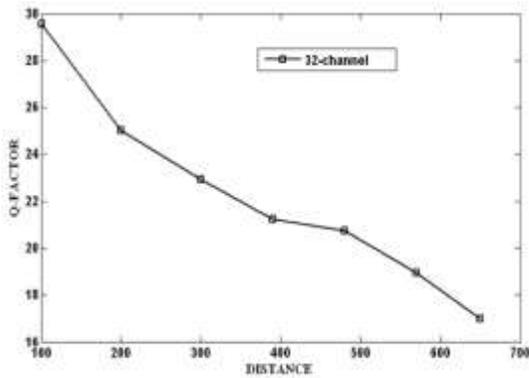
Figure 2: Quality factor vs. distance for 32 channels
