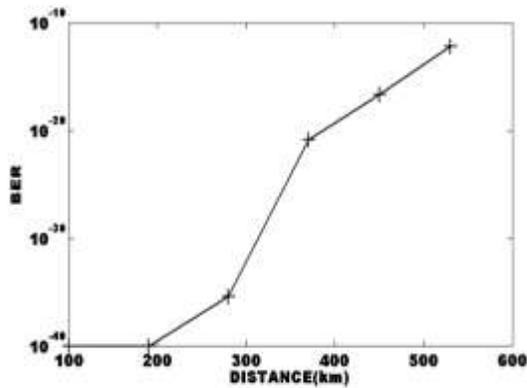
Figure 6: BER vs. distance for 64 channels
