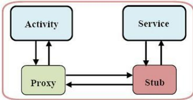
Fig.1. An overview of the Android IPC mechanism
