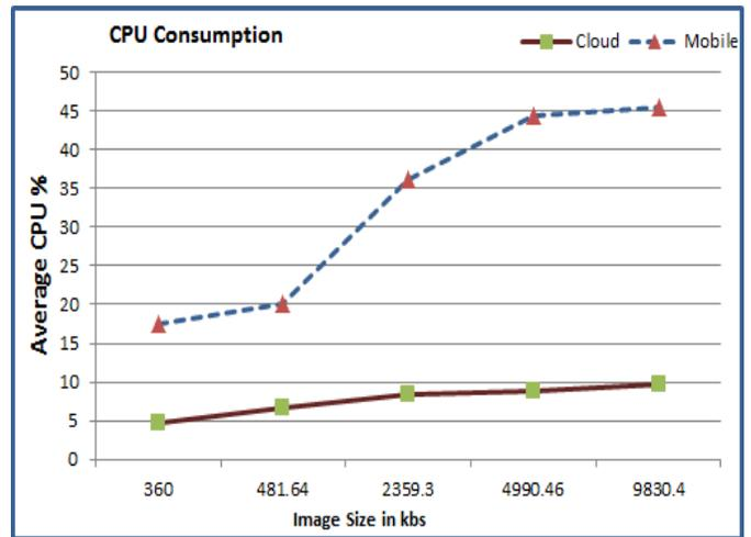
Fig.6. CPU consumption percentage on mobile and on Cloud
