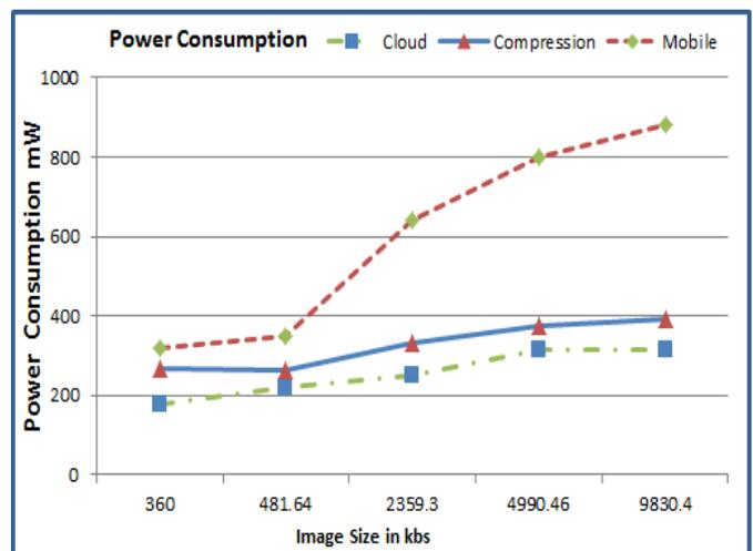
Fig.11. Power Consumption of the application under the three scenarios using low bandwidth network
