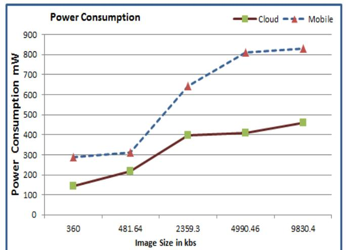
Fig.7. Power consumption on mobile and on Cloud
