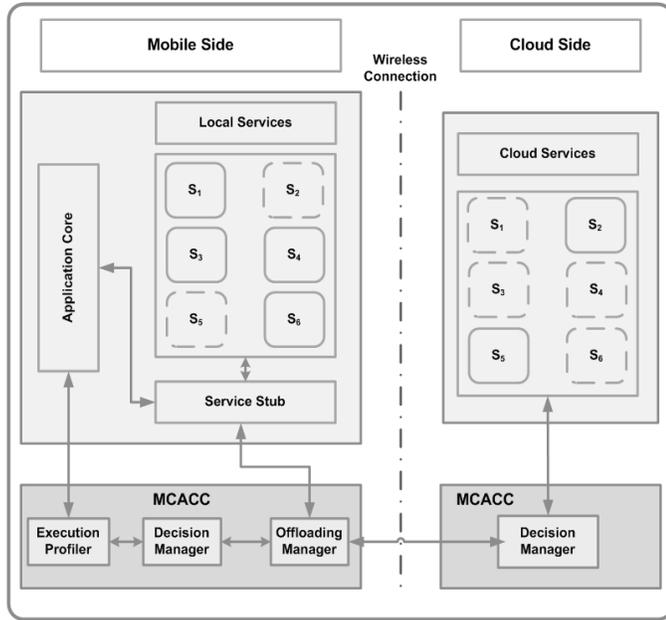
Fig.2. MCACC Architecture – services like S2 can be offloaded to run on the Cloud using Offloading Manager and Cloud Manager.
