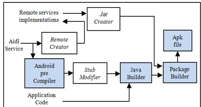
Fig.3. A schematic overview of how components integrate into the default build process.
