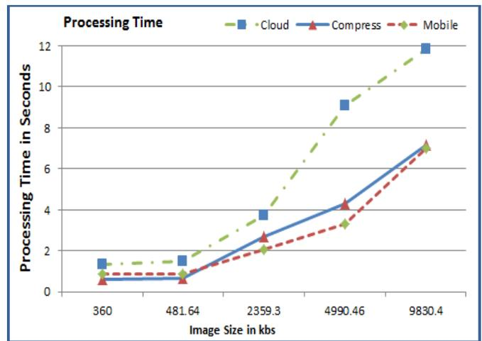
Fig.9. Processing Time of the application under the three scenarios using low bandwidth network
