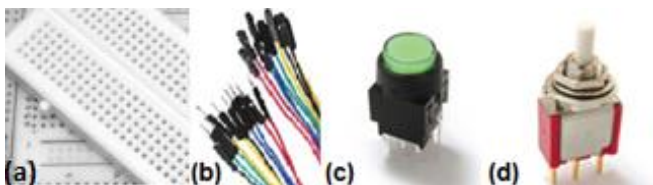
Fig. 7. Images of Some of the Hardware Parts used in Designing the Interactive Keypad : (a) Breadboard, (b) Jumper Caples (c) Latching Push Button Switch (d) Button [16].
