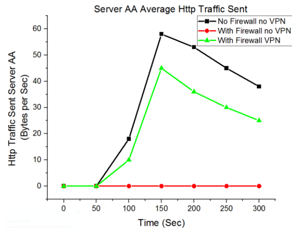
Fig. 14. Simulation Result of Server AA Average http Traffic Sent for No Firewall No VPN, with Firewall No VPN and with Firewall VPN.
