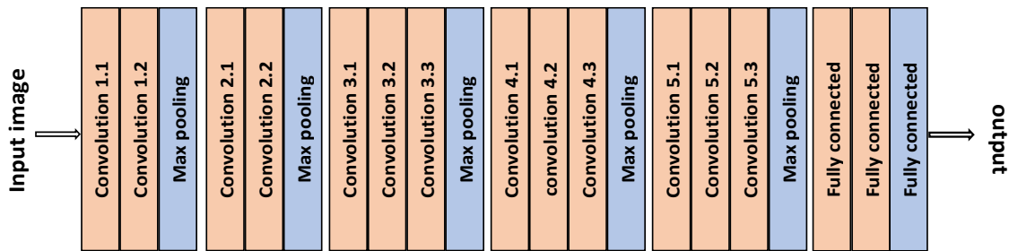
Fig. 4. A schematic of VGG-16 architecture.
