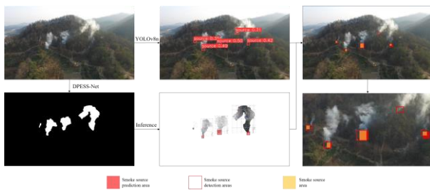
Fig. 4. Schematic diagram of smoke source localization method.
