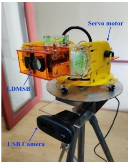
Fig. 3. Laser distance measuring functional testing equipment.
