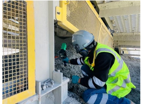
Fig. 10. The inspector comparing the temperatures in an idler roller.
