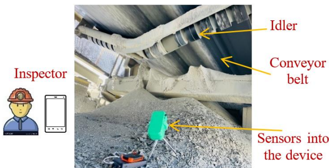
Fig. 1. The prototype installed in “MMG Las Bambas” mining company (Peru).
