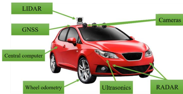
Fig. 1. AVs and sensor technology for intelligent transportation.
