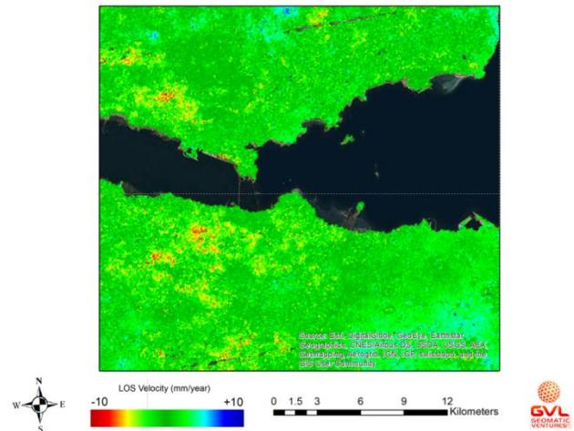
Fig. 18. InSAR image processing of the Sanqi Bridge (October 2017).
