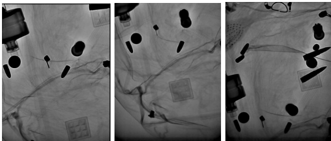
Fig. 2. Some samples of the X-ray images after ammunition detection: First row, 9 mm handgun bullets, AK-47 Machine gun bullets, and the 12-Gauge shotgun shells. Second row, resultant binary images.
