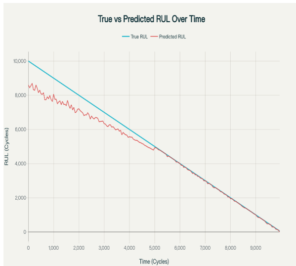
Fig. 4. True RUL vs. Predicted RUL by the hybrid model over time.
