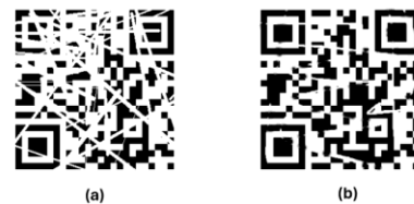
Fig. 5. Image showing the reconstruction of missing parts in a QR code using the GANs + SN technique: (a) Damaged QR code, not scannable; (b) GANs + SN reconstruction, scannable.
