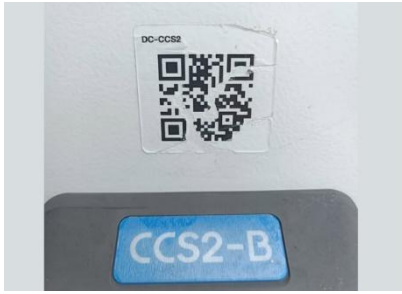
Fig. 1. An example of a damaged QR Code on an EV charging station at a gas station.
