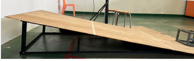
Fig. 5. The experimental testbed (2.4 m × 1.2 m), shown in its inclined configuration.
