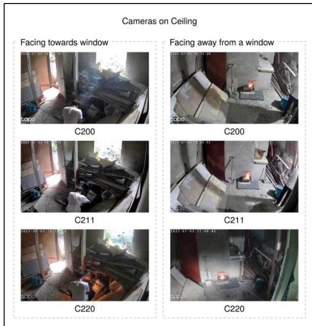
Fig. 10. Fire detection frames from ceiling-mounted cameras.
