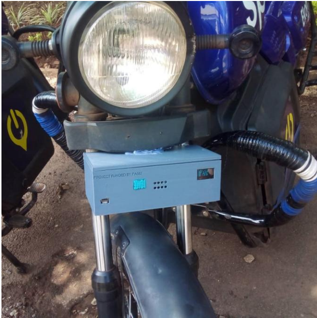
Fig. 18. Clean city IoT device mounted on motorcycle.
