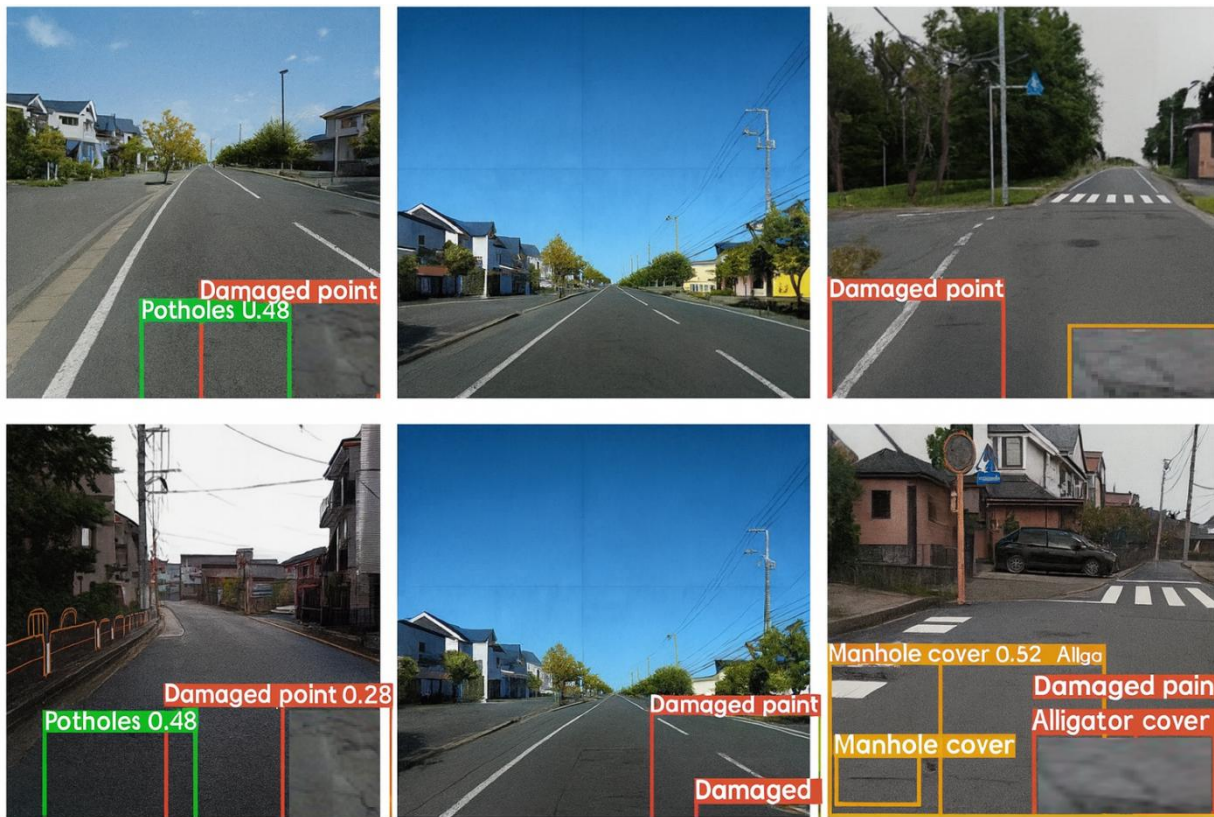
Fig. 5. Qualitative road damage detection results produced by the proposed multi-scale ROI-aligned framework across diverse roadway scenes.
