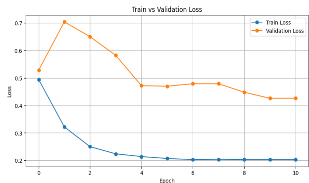
Fig. 4. The train and validation loss results for YOLOv5.
