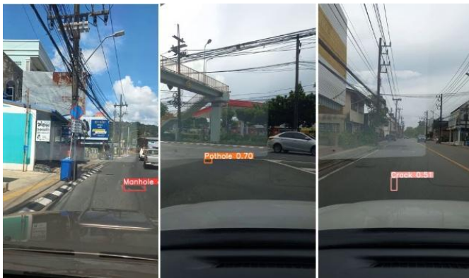
Fig. 9. Three examples when detected by RoadSCnet model.
