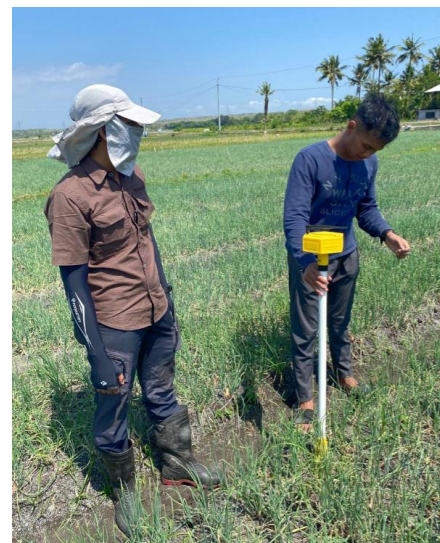
Fig. 1. In-situ soil NPK data acquisition and GNSS-based georeferencing during field sampling.
