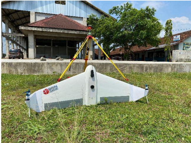
Fig. 2. Fixed-wing UAV platform used for high-resolution RGB image acquisition.
