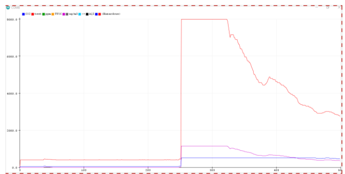
Fig. 2. Sample TVOC and CO 2 signal change over time when exposed to a TVOC.
