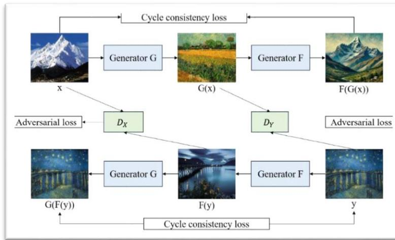
Fig. 1. ConvNeXt-CycleGAN overall network structure diagram.
