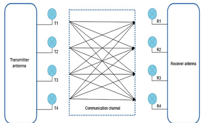
Fig. 1. Nakagami- $q$  Fading MIMO wireless channel system model.
