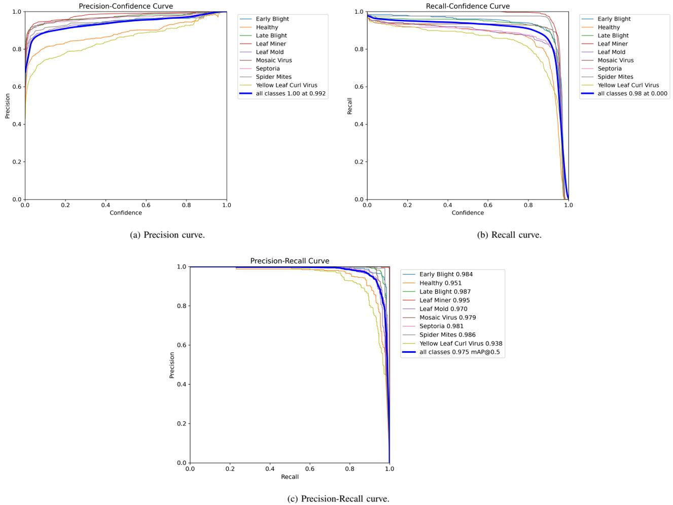
Fig. 8. Precision and recall for fine-tuned YOLOv8.
