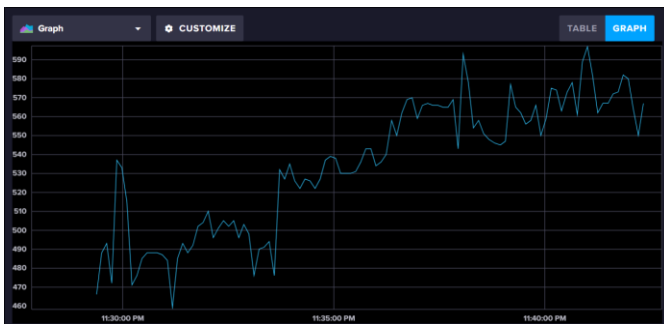
Fig. 8. Data collection of solar irradiance real-time value in graph.
