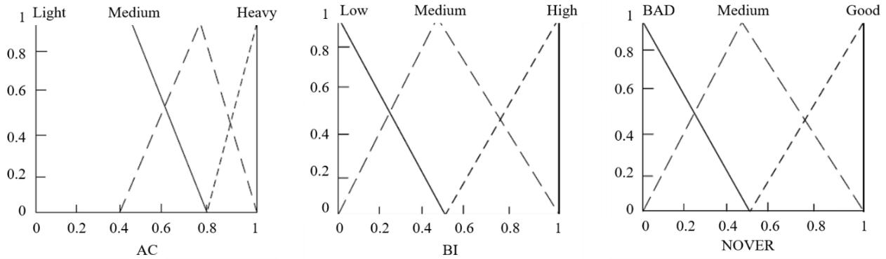
Fig. 3. Fuzzy membership functions for inputs.
