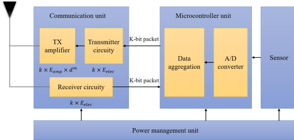
Fig. 1. Components and configuration of SNs in WSNs.
