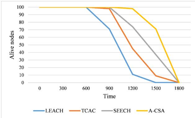
Fig. 5. Network lifetime comparison for first scenario.
