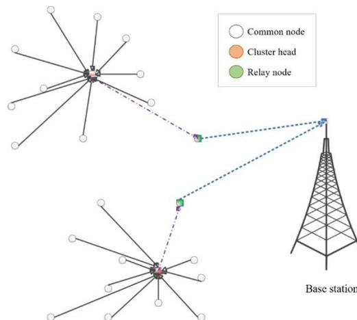
Fig. 2. Network architecture of the proposed protocol.
