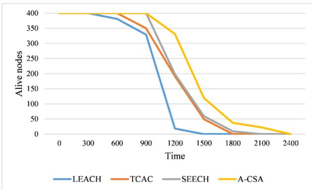
Fig. 6. Network lifetime comparison for second scenario.
