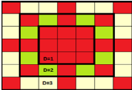
Fig. 4. 3x3 Filter with different dilation rate as 1, 2, and 3.
