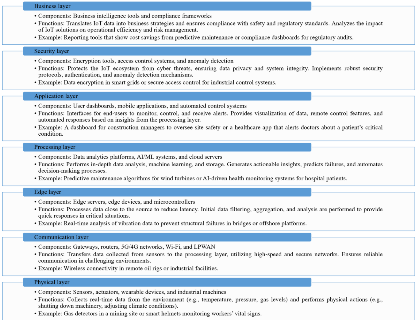
Fig. 2. Layered IIOT architecture explicitly designed for high-risk environments.
