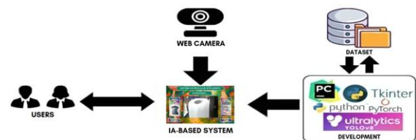
Fig. 3. Technological architecture for system development.
