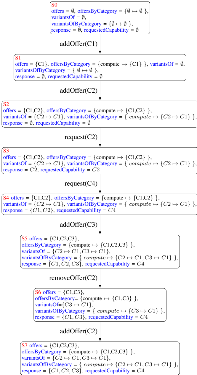
Fig. 14. State transition diagram of the cloud service discovery system under the validation scenario.
