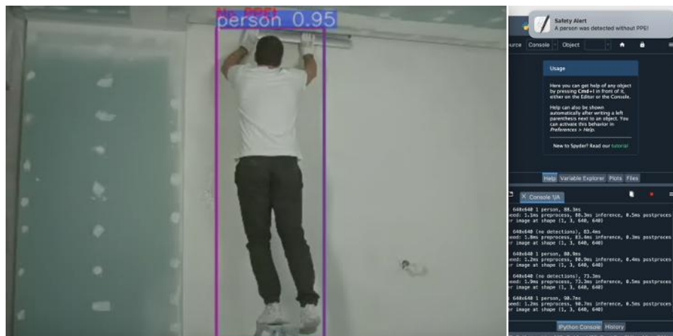
Fig. 8. Real-time detection of PPE compliance and safety violations.
