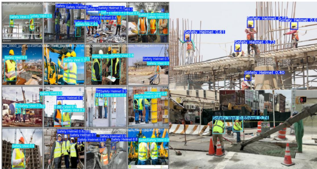
Fig. 7. Image evaluation: Training set dataset (left) and inference ran on prerecorded video data (right).
