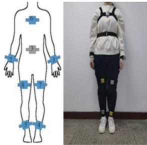
Fig. 7. Schematic diagram of multi-sensor arrangement for medical monitoring.
