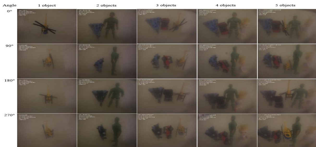
Fig. 9. Different angle of object setting for dataset for pond underwater images (depth from water surface is 20 cm, distance of object to camera is 30 cm).
