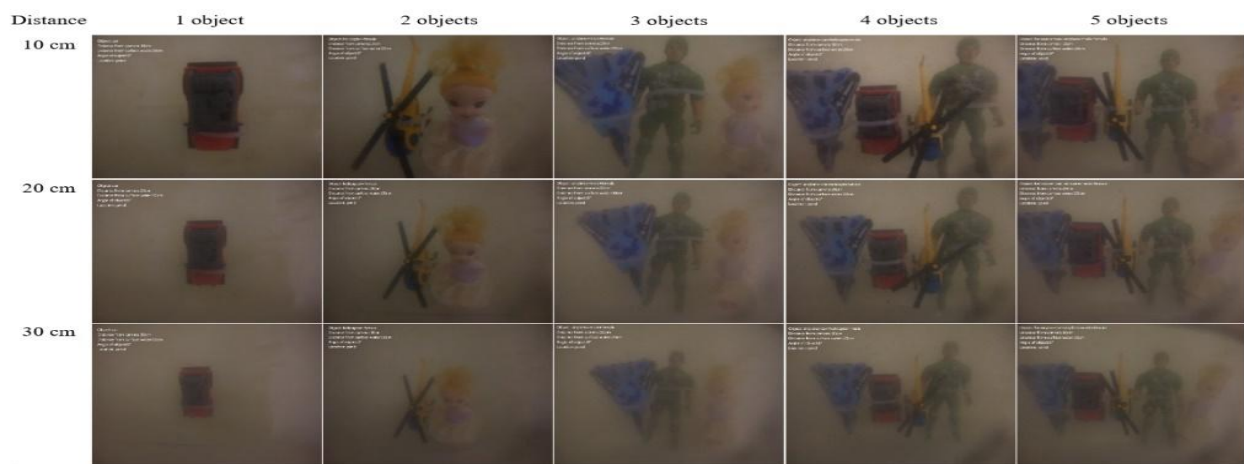
Fig. 8. Different camera distances from the object setting for pond underwater images (depth of water surface is 20cm and angle of object is 0 °).
