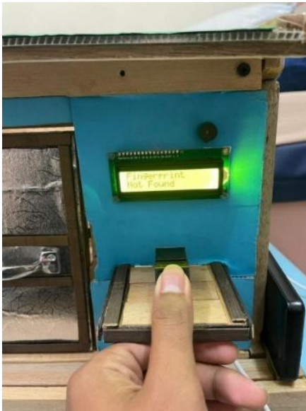
Fig. 10. Unauthorized user attempting access with an incorrect fingerprint.
