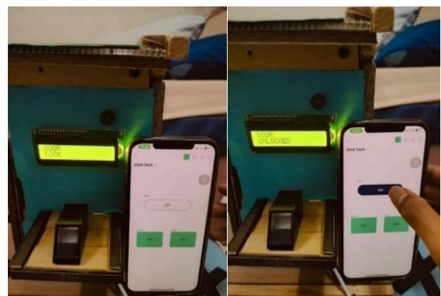
Fig. 12. Remote operation and control via Blynk.
