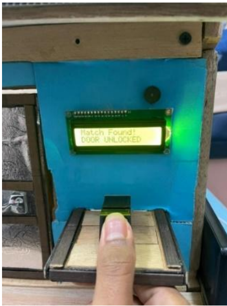
Fig. 9. Authorized user gaining access with a correct fingerprint.
