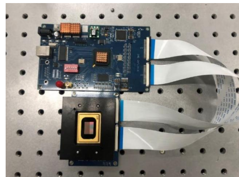
Fig. 7. Structure of DMD development board.
