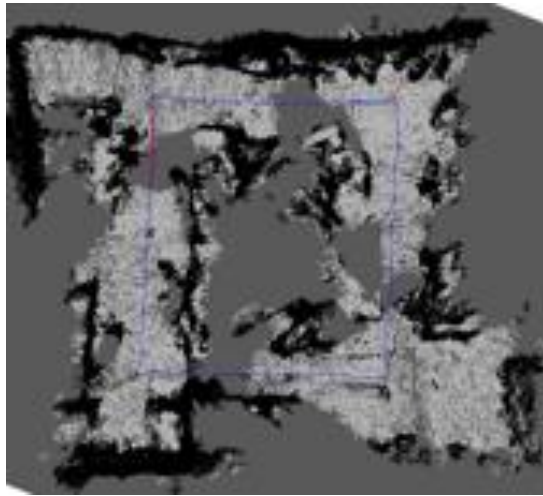
Fig. 7. Occupancy grid map of handheld mapping.
