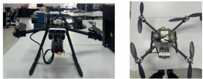
Fig. 1. Front view (left) and top view (right) of the assembled UAV.
