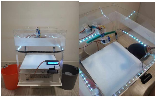
Fig. 11. Solid waste classification machine prototype.
