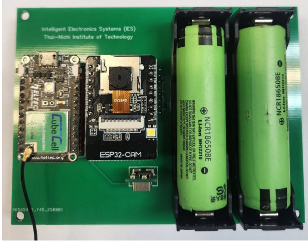
Fig. 2. Custom-designed embedded device of transmission node.
