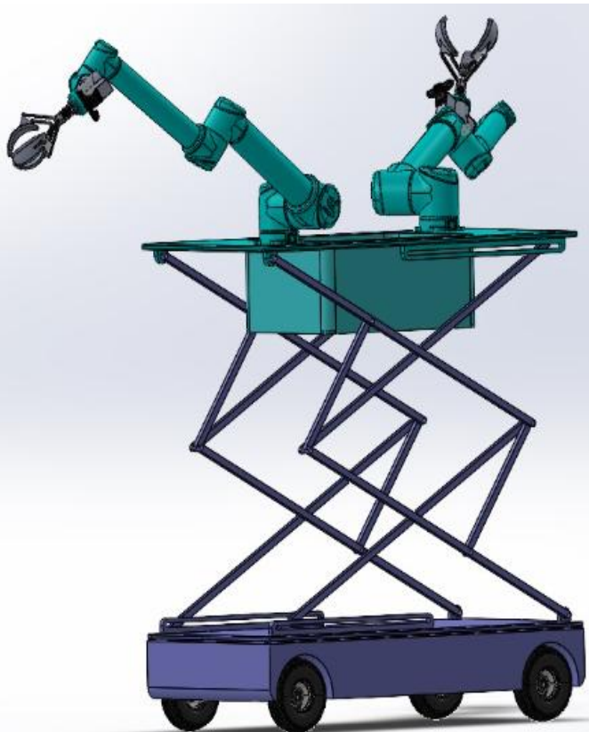
Fig. 6. Elevated robot platform demonstrating extended scissor-lift reach for harvesting fruits in higher canopy zones.
