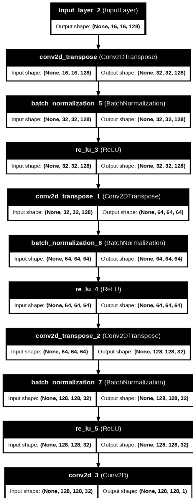
Fig. 4. This is a 2D decoder architecture for reconstructing the output image from the denoised latent features.
