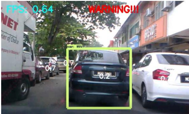
Fig. 15. Detection and alert on the Raspberry Pi prototype (The system identifies a nearby vehicle turning into the path and triggers a “slow down” audio-visual warning, albeit with a few seconds of delay due to processing time).
