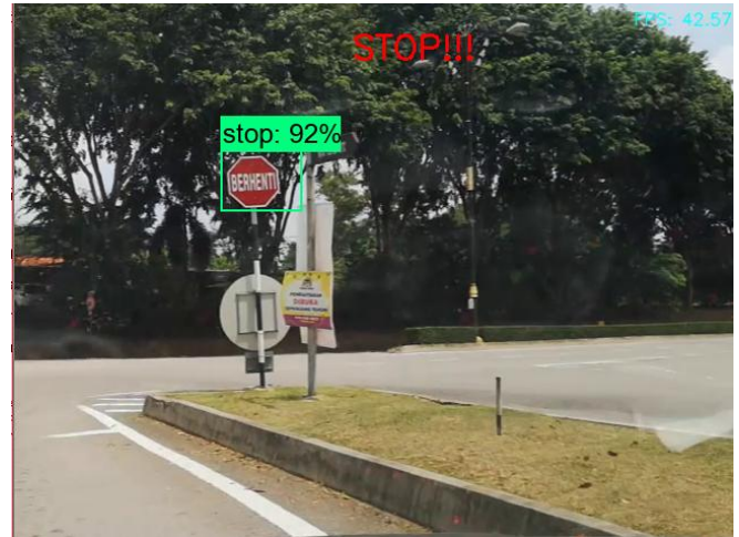
Fig. 5. Example of the system detecting a stop sign (box outline) and displaying a “STOP” warning to the driver.
