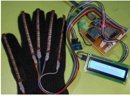
Fig. 3. Fully assembled smart-glove hardware prototype.
