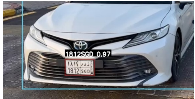
Fig. 12. License-plate recognition result for the selected frame, correctly decoding the plate number 1812SGD with a confidence score of 0.97.
