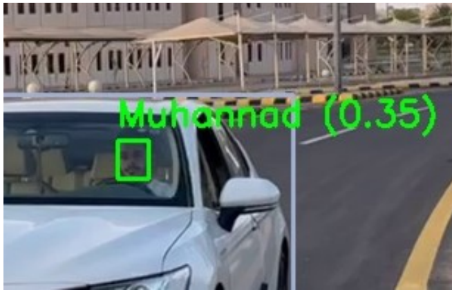
Fig. 13. In-vehicle face detection and recognition result, identifying the enrolled driver (Muhannad) with a confidence score of 0.35.
