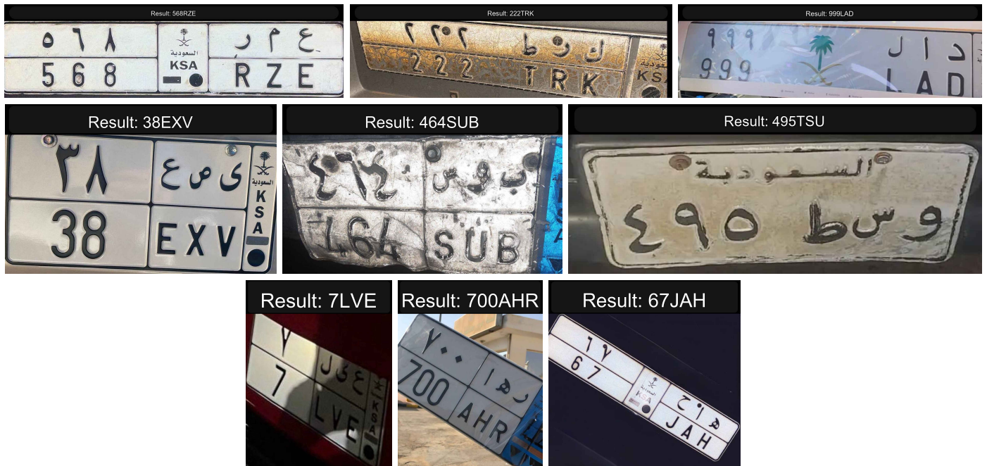
Fig. 5. Samples from the Saudi license-plate recognition dataset (35,000 images) encompass a diverse range of backgrounds, lighting conditions, scales, viewpoints, and official plate types. LPRNet predictions are shown above each plate.
