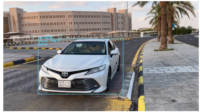
Fig. 11. Output of the vehicle make-model classifier, correctly identifying the car as a Toyota Camry with a confidence score of 0.9417.
