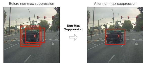
Fig. 3. Illustration of non-maximum suppression (NMS) removing overlapping bounding boxes and keeping only the highest-confidence detection per vehicle.
