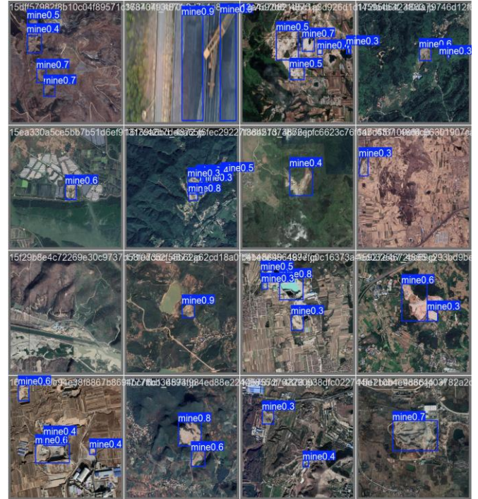
Fig. 14. Validation batch prediction samples showing bounding box localizations and confidence scores.
