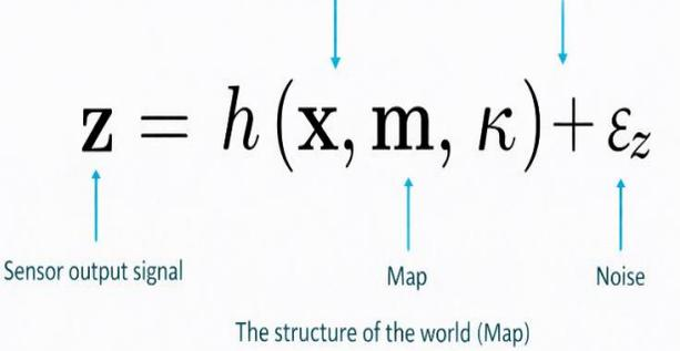
Fig. 6. Probabilistic Measurement Model Relating Sensor Observations, Robot State, Map, and Calibration Parameters
