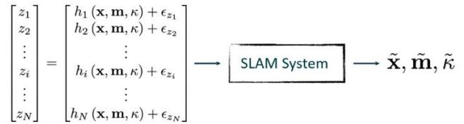
Fig. 7. Nonlinear SLAM Estimation Framework for Joint Optimization of State, Map, and Calibration Variables
